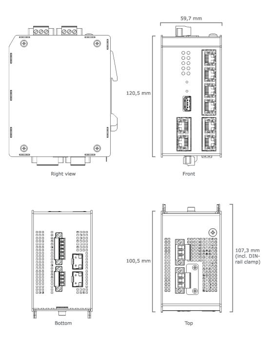
Height:120.5 mm (Without connectors)Width:59.7 mmDepth:100.5 mm (107.3 mm incl. DIN-rail holder)
